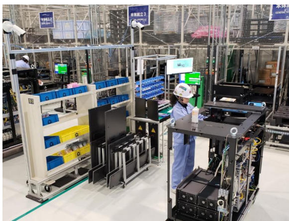
Assembly Navigation System constructed at AMADA Fujinomiya Works
